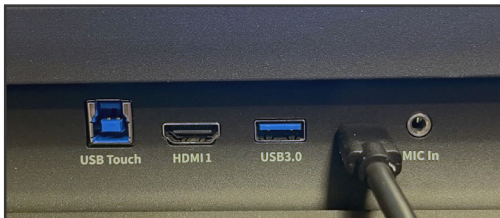
Front Ports with USB Type-C cable connected.
